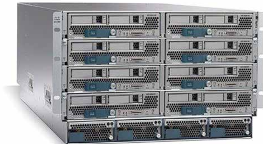
Figure 6 : UCS 5100 Blade Server Chassis
