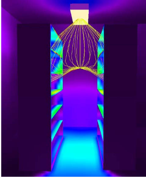
Figure 7: Traditional fluorescent light
