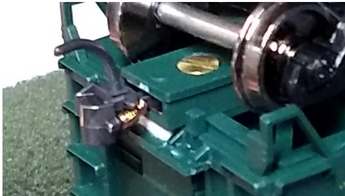
This photo shows a piece of white styrene used as reinforcement for the walkway on the green car.
